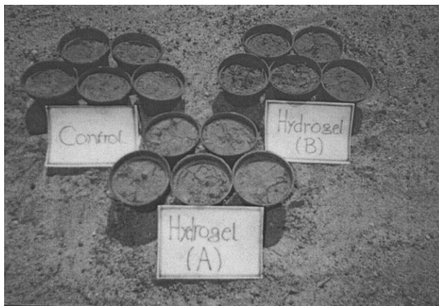
Figure 11 The properties of compact clay soil containing (A) 1 g PAAm/PAAcK and (B) 2 g PAAm/PAAcK.
